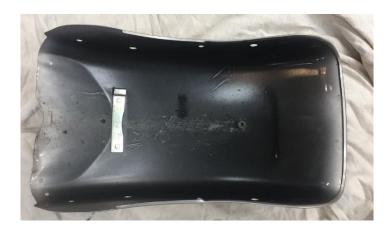
Attach new licence plate surround to the fender eliminator licence plate backing with a cable tie as shown below, to temporarily secure in place (not applicable for WA/SA/NZ or Euro/UK models).
