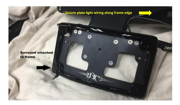
Using supplied cable ties, secure new LED plate light wiring to provisions along the edge of fender eliminator frame, as shown above.
